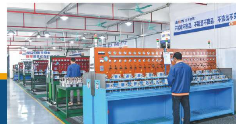
润滑泵测试 Lubrication pump test
